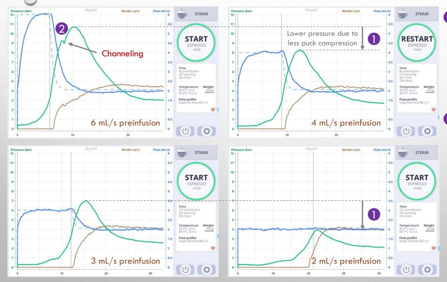
With the same grind size and targeted flow rate for the extraction phase, decrease the preinfusion flow rate reduces puck compression with direct impact on the maximum pressure reached during extraction (flow profile)
