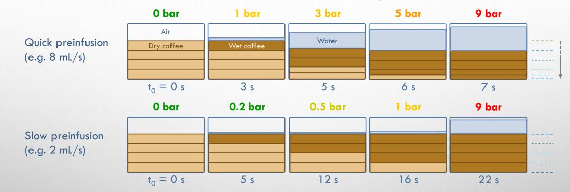
• During preinfusion with a quick pressure increase the bottom layers of the puck are more compressed
